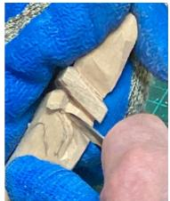
V-cut – point of knife in one way, turn wood and cut back.
