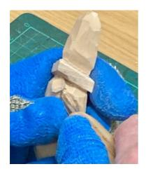
Stop cut – cut straight in to the wood to form a 'stop' or end, up to which you can do a push cut.
